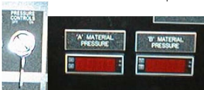
**NOTE:** Pressure readouts set for high set point, if the pressure rises above the set point the audio alarm sounds and the red light on the light tower illuminates until the clear pressure fault pushbutton is pressed.
